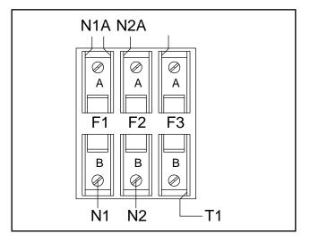
Figure 10. Transfer Switch Fuse Block
